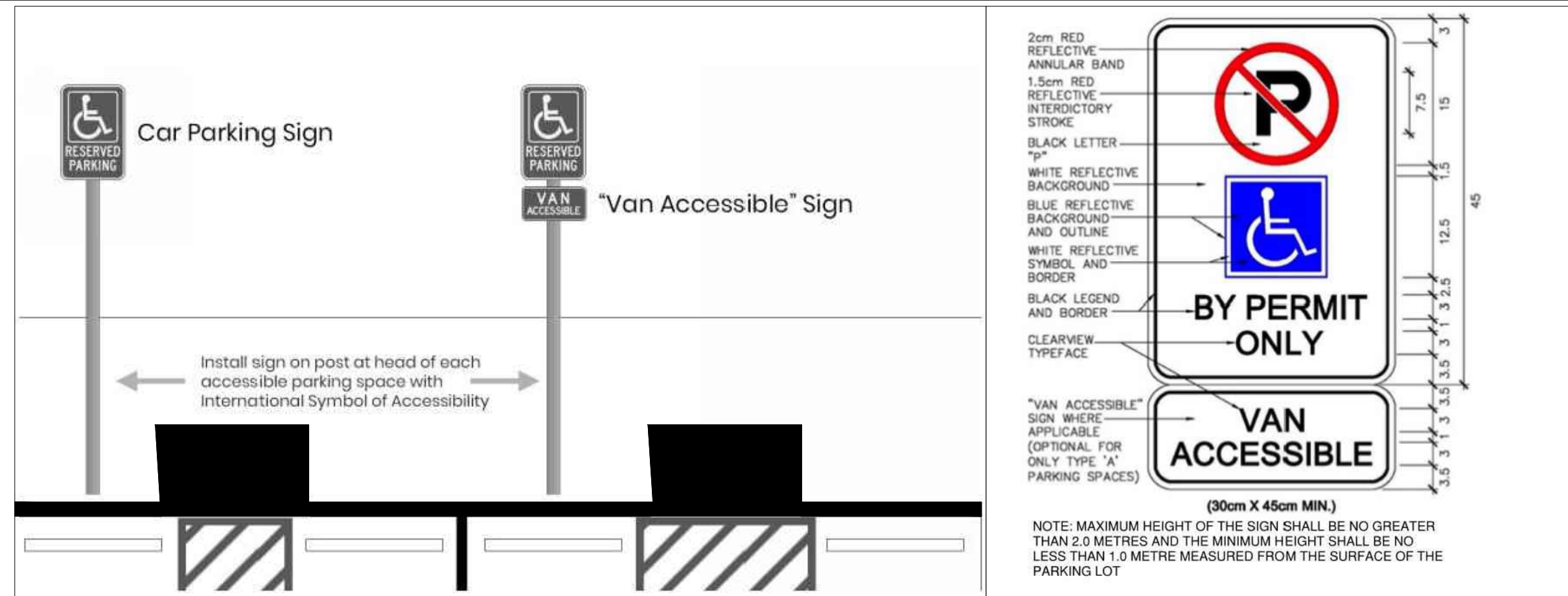
ACCESIBLE PARKING SIGNAGE AND LOCATION 6 SCALE: N.T.S.
